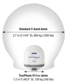
85% smaller in volume and lighter than standard C-band antennas, TracPhone V11HTS is faster, easier, and less expensive to install.
